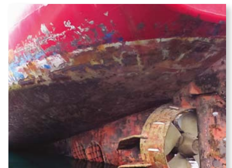
Three photos of the hull of RRS Ernest Shackleton showing the condition of the paint (conventional ice paint and corresponding repair coating) before Ecospeed was applied.
