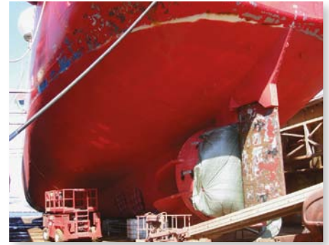
Three comparison photos of similar areas of the hull after the switch to Ecospeed underwater hull coating system and two seasons of sailing in the ice. Note that the boot top and rudder, seen to have suffered damage in the photos on the right, were not coated with Ecospeed in 2009 along with the rest of the underwater hull. This has now been remedied in 2011.
