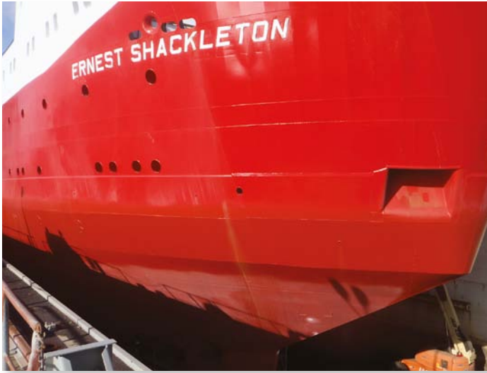
Newly Ecospeed coated boot top area above the water line
