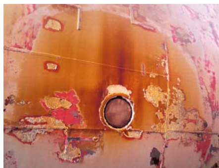
Three photos of the hull of RRS Ernest Shackleton showing the condition of the paint (conventional ice paint and corresponding repair coating) before Ecospeed was applied.
