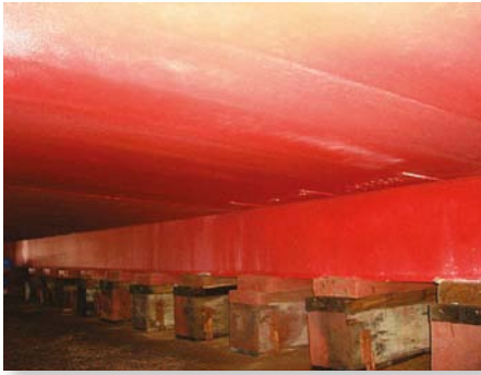
Three comparison photos of similar areas of the hull after the switch to Ecospeed underwater hull coating system and two seasons of sailing in the ice. Note that the boot top and rudder, seen to have suffered damage in the photos on the right, were not coated with Ecospeed in 2009 along with the rest of the underwater hull. This has now been remedied in 2011.
