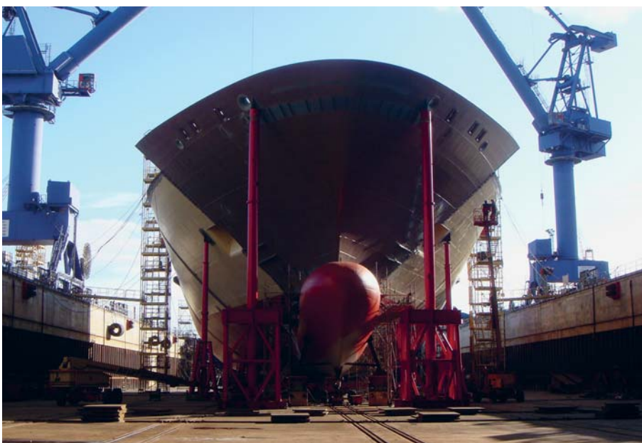
The underwater hull of the largest ROPAX ferry in the world is given an Ecospeed protective coating
