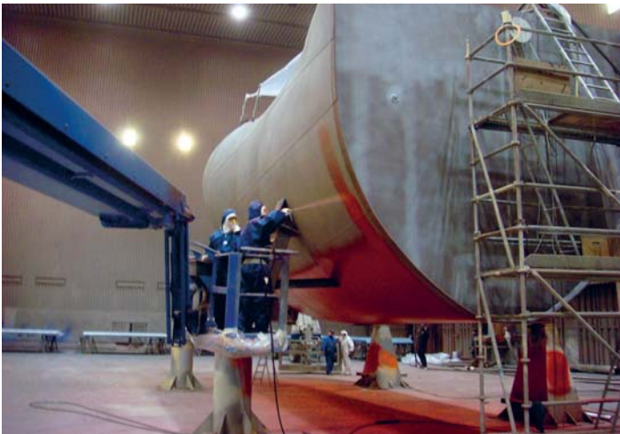
Ecospeed application on bulbous bow of ROPAX ferry...
