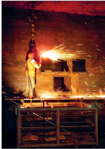
Cutting away damaged area on side shell plating of tanker
