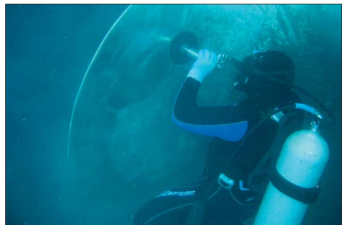
Hydrex diver during propeller blade polishing
