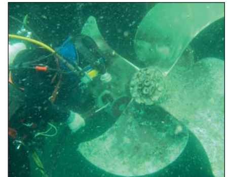
Hydrex diver polishing propeller blades
