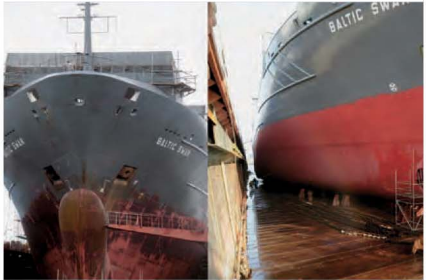
Comparison of the same container ship with a conventional biocidal antifouling (left) and Ecospeed (right) after spending a period of 2.5 years operating in the Baltic Sea
