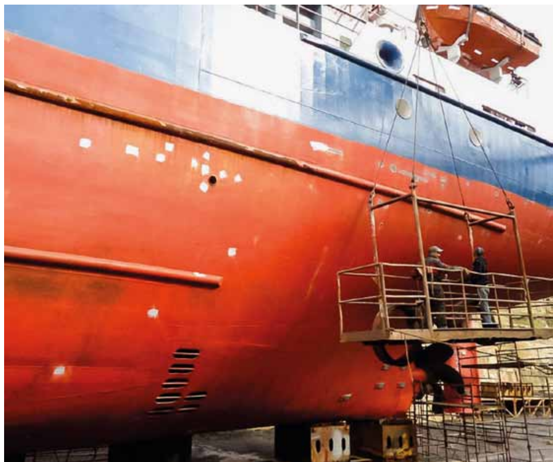
Minor touch-ups to the Crownbreeze in drydock in 2012 after five years of service since applying the Ecospeed coating.
