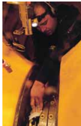
Dry underwater stern tube seal repair inside flexible mobdock.
