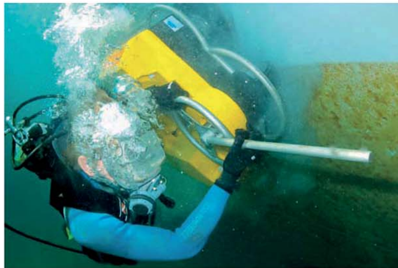
Ecospeed coated hull being cleaned of slime using a Hydrex medium-sized, self-propelling in-water cleaning tool
