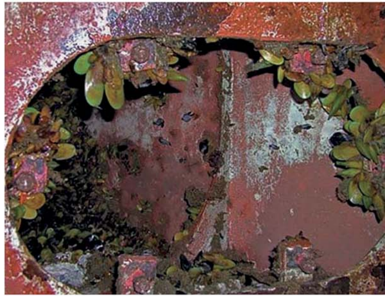
A "niche area" of a hull coated with biocidal antifouling paint
